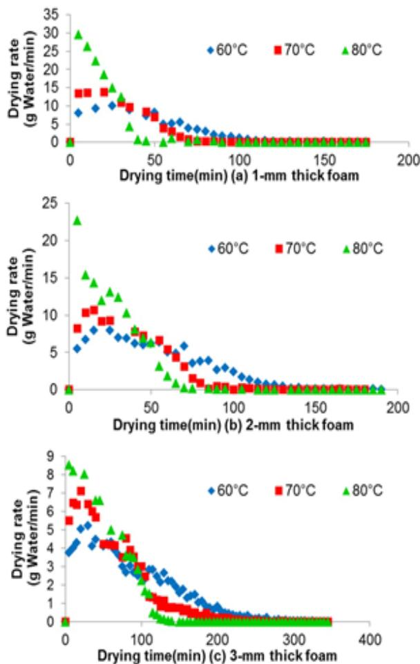
Figure 1. Drying rate of passion fruit aril foam at (a) 1-mm (b) 2-mm (c) 3-mm at different drying temperatures
